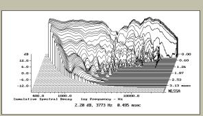
Fig.10 Audio Physic Scorpio, cumulative spectral-decay plot at 50" (0.15ms risetime).
