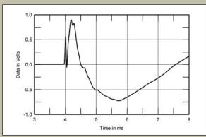
Fig.9 Audio Physic Scorpio, step response on tweeter axis at 50" (5ms time window, 30kHz bandwidth).
