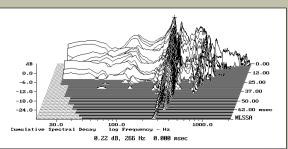
Fig.2 Audio Physic Scorpio, cumulative spectral-decay plot calculated from the output of an accelerometer fastened to the cabinet's front baffle level with the woofers (MLS driving voltage to speaker, 7.55V; measurement bandwidth, 2kHz).
