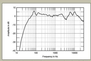
Fig.5 Audio Physic Scorpio, anechoic response on axis 43" from the floor at 50", averaged across 30° horizontal window and corrected for microphone response, with the complex sum of the nearfield driveunit responses.
