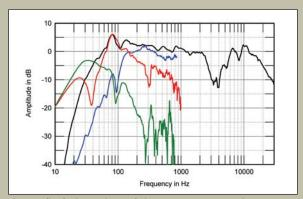
Fig.3 Audio Physic Scorpio, anechoic response on tweeter axis at 50", averaged across 30° horizontal window and corrected for microphone response, with the nearfield responses of the midrange units (blue), woofers (red), ports (green), and their complex sum (black).
