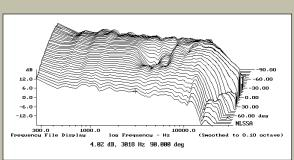
Fig. 7 Audio Physic Scorpio, lateral response family at 50", from back to front: responses 90–5° off axis, tweeter-axis response, responses 5–90° off axis.
