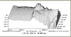
Fig.8 Audio Physic Scorpio, lateral response family at 50", normalized to response on tweeter axis, from back to front: differences in response 90–5° off axis, reference response, differences in response 5–90° off
