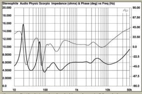
g.1 Audio Physic Scorpio, electrical impedance (solid) and phase (dashed). (2 ohms/vertical div.)
