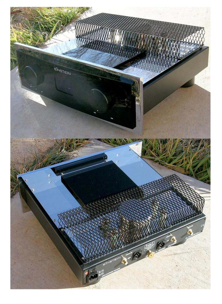
Removal of the tube cages is child's play on both integrated and CDP and merely involves the loosening of 4 hex bolts. Still, be careful not to push the spacers between the black chassis and the floating mirror cover into the component or
