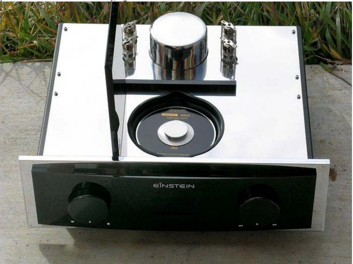
The CDP's acrylic flip lid reveals a deep well with finger spaces in the 12:00 and 6:00 o'clock positions, rubber edge-banding to buffer the lid from the mirror-gloss top, a magnetic puck and a non-suspended hard-mounted laser assembly.
