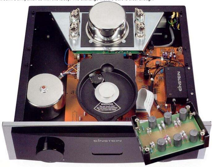
The CDP's transport is Rega-based while the analog reconstruction filter is a zero-opamp purely passive resistor/coil affair [insert above] for shallow filtering. This feeds into the quartet of paralleled double-triode 6922s in the output stage. Output impedance is 51 ohms and dynamic range 101dB. The XLR outputs aren't truly balanced and thus not a performance but convenience option [the matching *The Tube* linestage is a fully symmetrical unit from input to output, however].
