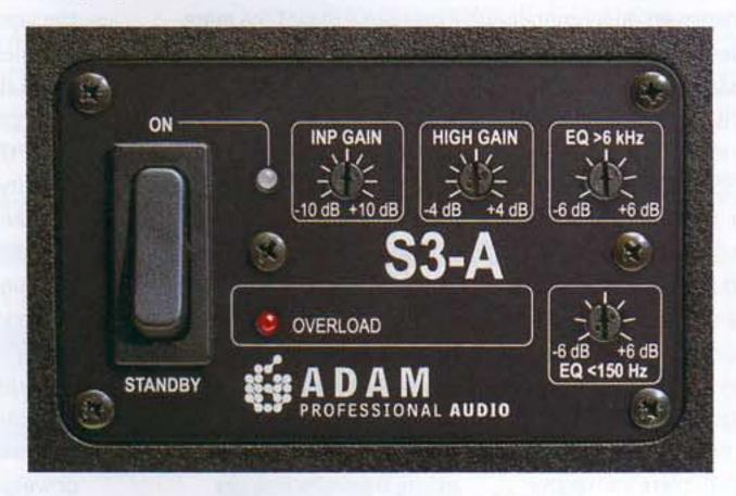
heat sink, an IEC mains inlet and a power switch. The signal comes in on a balanced XLR. Frequency adjustments are made via the four slotted rotary controls on the panel above the tweeter, where the input sensitivity can be tweaked by ±10dB and the tweeter gain can be adjusted over a ±4dB range. The two remaining controls provide ±13dB of room EQ at 6kHz and 140Hz, though I conducted my review with all frequency tailoring screws set flat and had no cause to adjust them.
